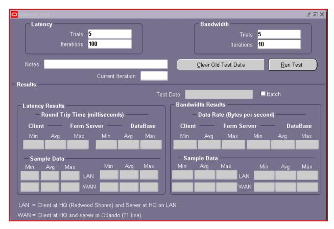
For every iteration a single packet is sent from the client application to the server and back to server from client.
