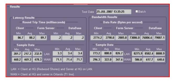
Latency Results display the minimum, average, and maximum round trip time for a single round trip from a PC client to the server.
