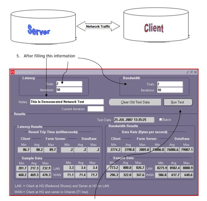
6. Select the Run Test button to perform the test.
